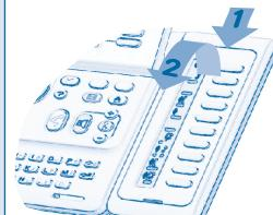
An extension unit can be fitted to your telephone. This provides additional keys which can be configured as function keys, line keys, call keys, etc.
